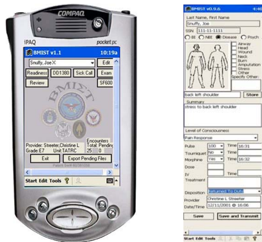
Figure 6: The BMIS-T, shown at left, is a handheld system that will allow capture of medical encounter information by far-forward medics. A sample display screen is shown at right.
